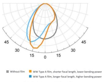
Measured light distribution curve, WW Type A film
